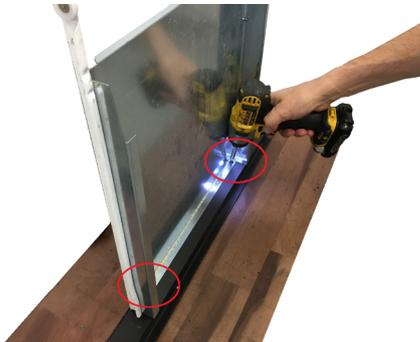
**Fig. 36 - Demontage Frontplatte**
